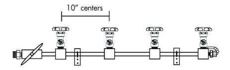
The Inlet Header manifold is supplied pre-assembled with the exception of the two (2) mounting "L" brackets *GMF-3611* and mounting hardware supplied in a separate box.
