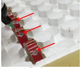
**Figure 7** Location where the adhesive is applied
