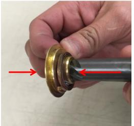
Figure 1 Remove the sharp edges from the center hole on both sides using the edge deburring tool
