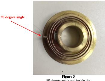
90 degree angle and inside the outer diameter
