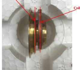
**Figure 2** Coil is parallel with the InGage body
