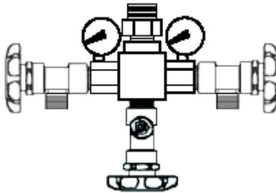
1. Thread 2 each **1131-0000** Orifice Quick Vac onto each side outlet of **GMF-3041** cross joint.
