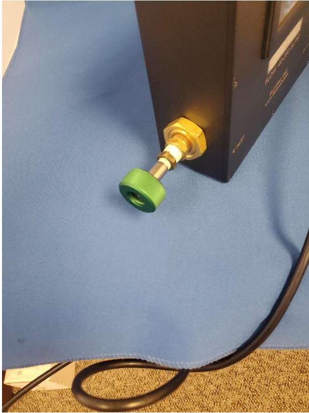
Power and Flow Outlet Connections.
