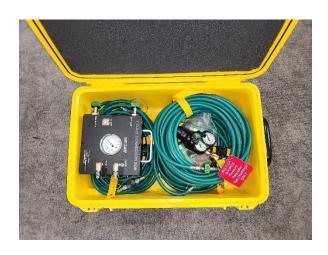
Do not interchange the flowmeters from one strand to another. They are sized for a total flow of less than 75 LPM/strand and interchange of flow meters of a higher flow could cause the regulator to be overloaded, resulting in loss of flow to the patient.
