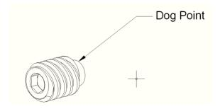
Step 5) Install the two Flat Point set screws. It is important to assemble the dog point set screws first. The Flat Point Set Screws are for locking the Dog Point Set Screws. Check the assembly for smooth operation, no wobble when turned and no movement of the knob on the stem when operated.
